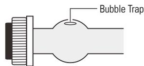
5. Place the test tube into the sample chamber. Note, the bubble trap is upward.
