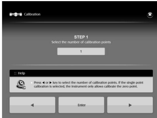
4. Make sure that remove the test tube from the sample chamber. Tap the ◀ or ▶ key until the visual field appears uniform brightness, tap the **Enter** key to confirm. Zero-point calibration is completed.
