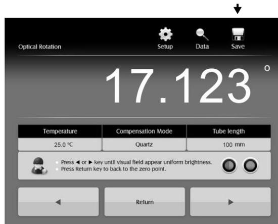
1.2 The default sample name is SAMPLE. If you need to modify, tap the ◀ key, then tap the letter keys to enter the new sample name. Tap the **Enter** key, the measured value will store into the memory.
