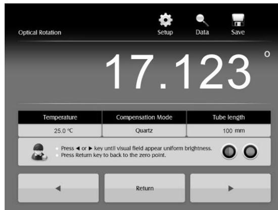
7. Tap the **Return** key, the instrument will automatically return to the zero-point. Measurement is completed.
