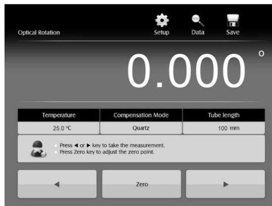
3. Tap the ◀ or ▶ key to adjust the instrument until the visual field appear the uniform brightness.
